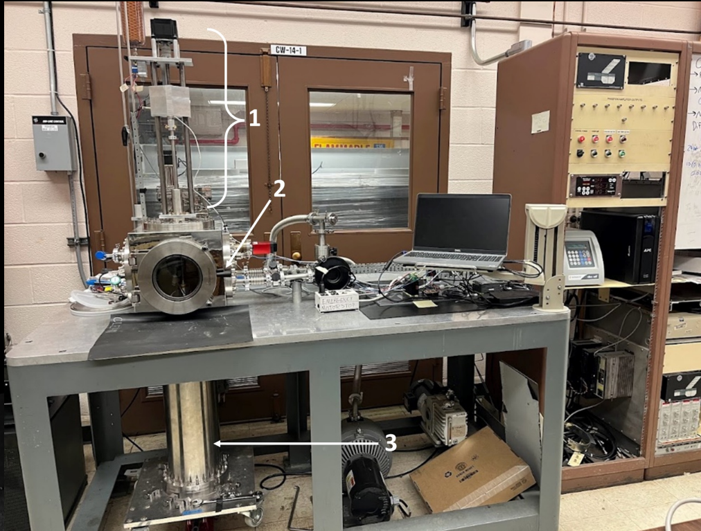
Figure 1. The CUBEvac experiment setup. 1) Penetration actuation stack, 2) Primary chamber volume where most sensors interface, and 3) Auxiliary chamber volume where the soil bin is located.
