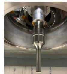
Figure 2. Resonant vibratory cylinder probe ( Sonics and Materials), 1.27 cm (0.5 in) diameter and 5.08 cm (2 in) from tip to beginning of fillet curve.
