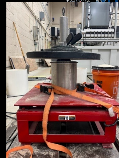
Figure 5. Soil preparation vibration table setup with a combined 34 kg of surcharge on the soil surface.
