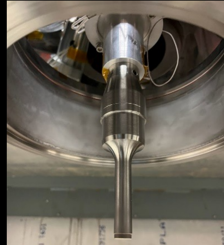
Figure 2. Cylinder probe from Sonics and Materials measuring 1.27 cm (0.5 in) in diameter and 5.08 cm (2 in) from the tip to the beginning of the fillet curve.
